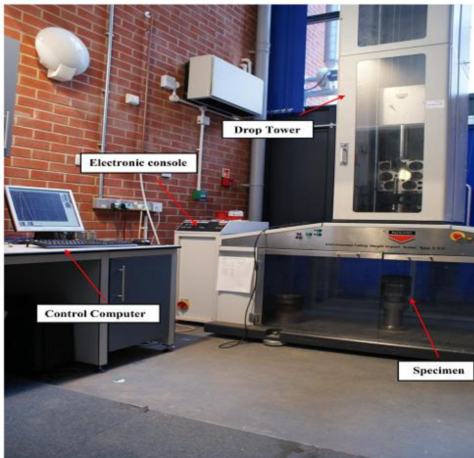
Figure 1 – Drop-weight type impact test device
